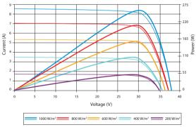
Excellent performance under weak light conditions: at an irradiation intensity of 200 W/m² (AM 1.5, 25 °C), 95.5% or higher of the STC efficiency (1000 W/m²) is achieved
